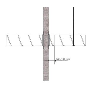
Distance from wall, deck or ceiling penetration to first duct joint must not be less than 100 mm.
